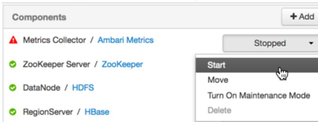
If you attempt to add a second Collector to the cluster without first switching AMS to distributed mode, the collector will install but will not be able to be started. To resolve this:
