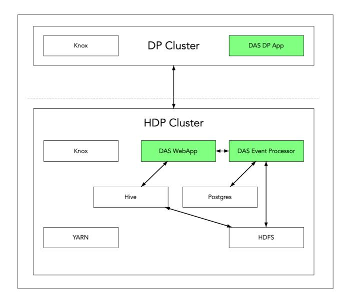
The DAS Webapp serves the DAS UI, and it should be on a machine that is accessible to your end users, or you should have a proxy setup to access the DAS UI.
