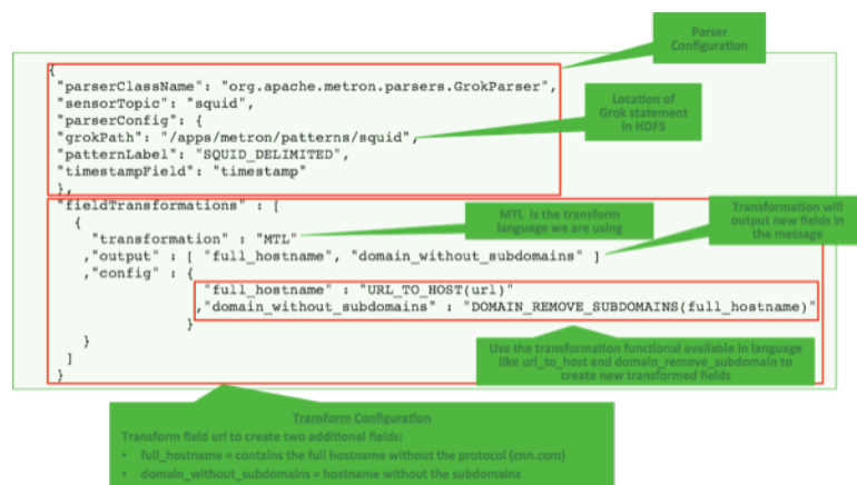
Figure 5.1. Configuration File with Transformation Information
