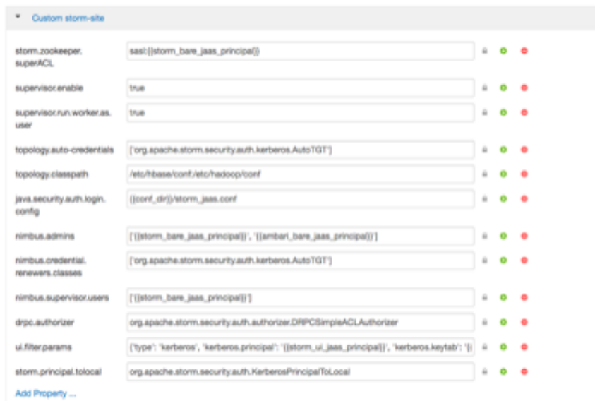
Figure 5.5. Final Custom Storm-site
