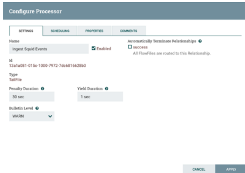
Figure 2.3. Configure Processor Dialog Box Settings Tab
