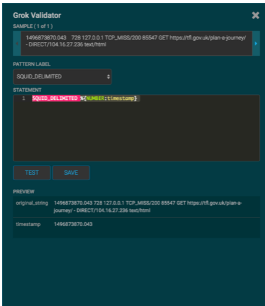
Figure 2.13. Grok Validator Panel with First Element and Test Results
