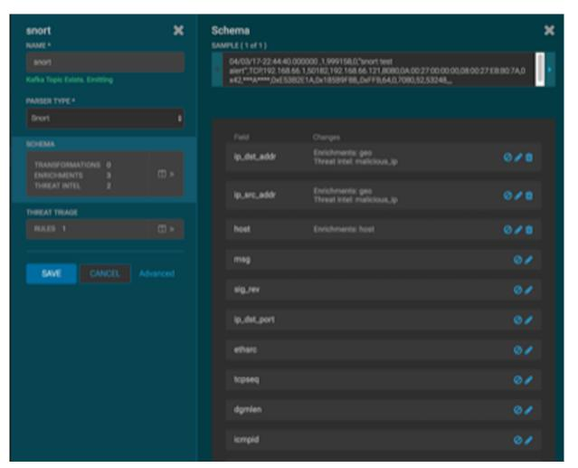
The Sample field displays a parsed version of a sample message from the sensor. The Management module tests your transformations against these parsed messages.
