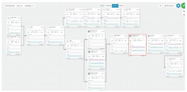
If you zoom in on the NORMALIZE-MODEL-FEATURES component, you will see that after the code change is made, throughput increases and the wait drops to 0.
