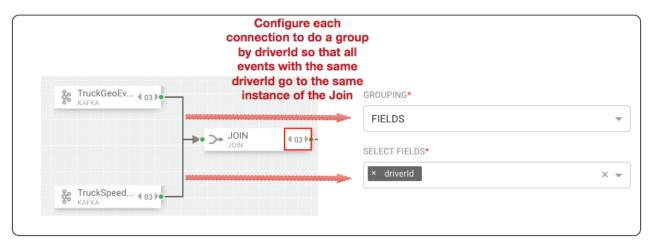
Increase the parallelism of the DriverAvgSpeed aggregate window from 1 to 3. Since the window groups by driverId,driverName and route, we can configure the connection to use fields grouping to send all events with those field values to the same instance of the window.
