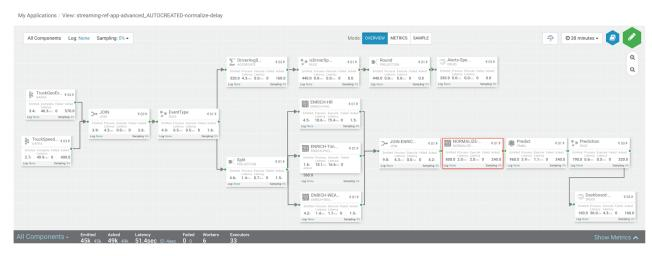
Scanning over the metrics, we see that the NORMALIZE-MODEL-FEATURES custom processor has high execute latency of 2 seconds. This means that over the last 30 minutes the average time an event spends in this component is 2 seconds.
