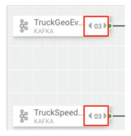
Increase the parallelism of the Join from 1 to 3. Since the join is grouped by driverId, we can configure the connection to use fields grouping to send all events with driverId to the same instance of the Join.
