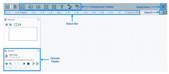
The Components Toolbar runs across the top left portion of your screen. It consists of the components you can drag onto the canvas to build your dataflow.
