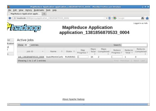
Details about the MapReduce process can be observed on the MapReduce Application page. Instead of Containers, the MapReduce application now refers to Maps and Reduces. Clicking the <code>job\_138</code>... link opens the MapReduce Job page:
