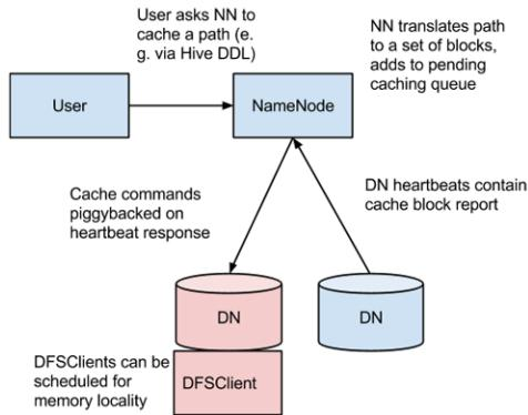
In this architecture, the NameNode is responsible for coordinating all of the DataNode off-heap caches in the cluster. The NameNode periodically receives a cache report from each DataNode. The cache report describes all of the blocks cached on the DataNode. The NameNode manages DataNode caches by piggy-backing cache and uncache commands on the DataNode heartbeat.
