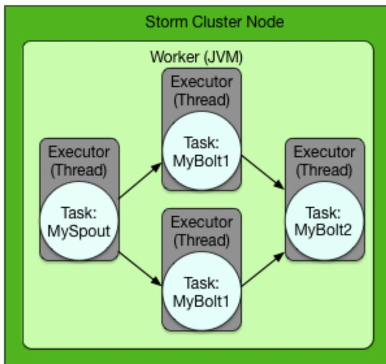
The number of executors is set at the level of individual topology components, so adding executors affects the code for the specified spouts and bolts. This differs from adding workers, which affects only the configuration of the topology.
