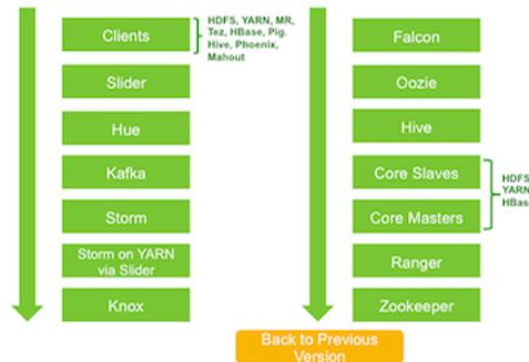
Here are the downgrade starting points based on your most recently upgraded component:
