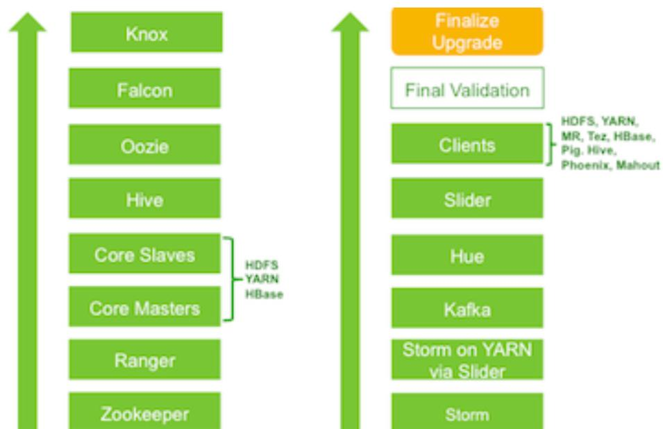
You will usually upgrade each component across all of its deployed nodes before upgrading the next component in the sequence. For example, first you'll upgrade Zookeeper across all nodes. Next you'll upgrade Ranger across all nodes:
