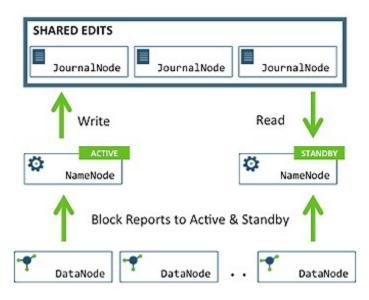
It is vital for the correct operation of an HA cluster that only one of the NameNodes should be Active at a time. Failure to do so, would cause the namespace state to quickly diverge between the two NameNode machines thus causing potential data loss. (This situation is called a **split-brain scenario**.)
