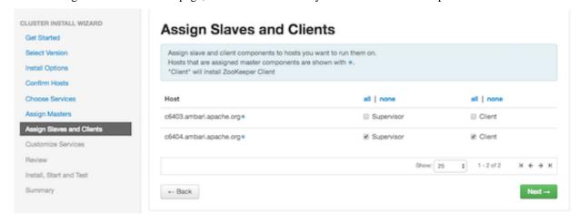
Storm supervisors are nodes from which the actual worker processes launch to execute spout and bolt tasks.
