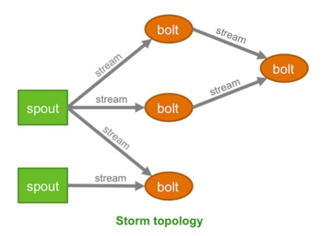
The TopologyBuilder class is the starting point for quickly writing Storm topologies with the storm-core API. The class contains getter and setter methods for the spouts and bolts that comprise the streaming data workflow, as shown in the following sample code.
