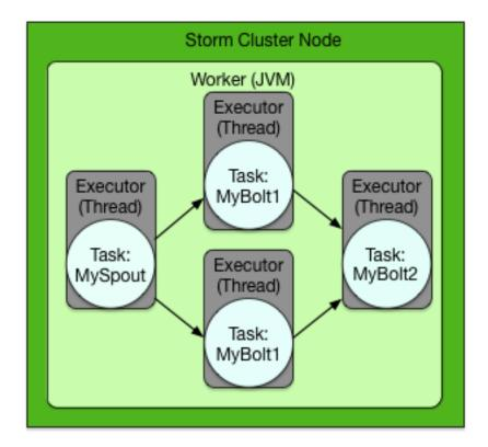
The number of executors is set at the level of individual topology components, so adding executors affects the code for the specified spouts and bolts. This differs from adding workers, which affects only the configuration of the topology.
