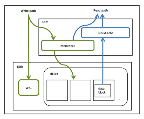
By default, BlockCache resides in an area of RAM that is managed by the Java Virtual Machine (JVM) garbage collector; this area of memory is known as on-heap memory or the JVM heap. The BlockCache implementation that manages the on-heap cache is called LruBlockCache.
