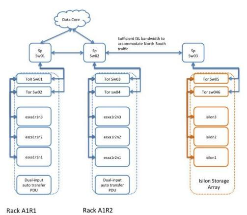
Note: In each rack of compute nodes, EMC recommends interspersing Isilon storage nodes connected to the respective ToR switches (if possible). For example, for two racks of compute nodes, distribute the Isilon storage nodes between the first and second rack, sharing the ToR switches. The Isilon storage nodes share an InfiniBand back end to provide better front-end performance (10 GB Ethernet).
