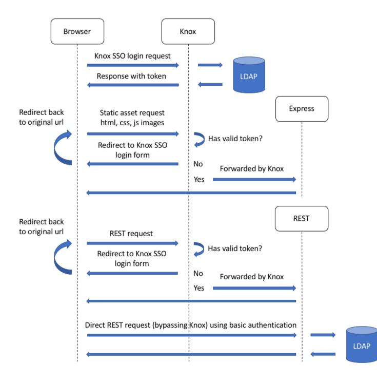
Note how the flow diagrams for Static asset requests and Rest requests (through Knox) are identical.
