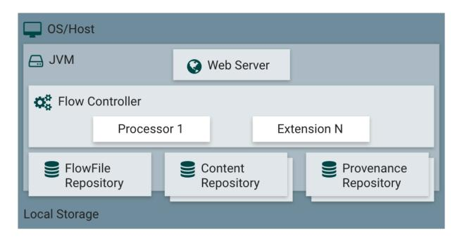
NiFi executes within a JVM on a host operating system. The primary components of NiFi on the JVM are as follows:
