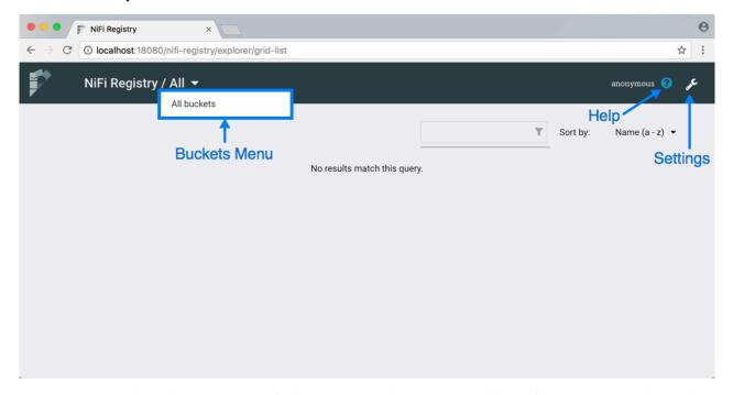
The Buckets menu is available at the top left of the screen. It allows the user to display flows based on which bucket
