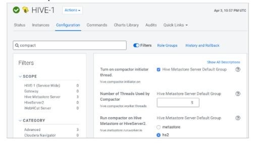
3. Check that Turn on Compactor Initiator Thread (hive.compactor.initiator.on), Number of Threads Used by Compactor (hive.compactor.worker.threads), and Run Compactor on Hive Metastore or HiveServer2 (hive.met astore.runworker.in) are set to the values shown above.
