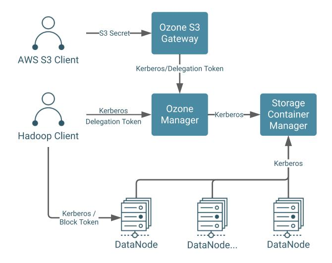
Each service must be configured with a valid Kerberos Principal Name and a corresponding keytab file, which is used by the service to login at the start of the service in secure mode. Correspondingly, Ozone clients must provide either a valid Kerberos ticket or security tokens to access Ozone services, such as OM for metadata and DataNode for read/write blocks.
