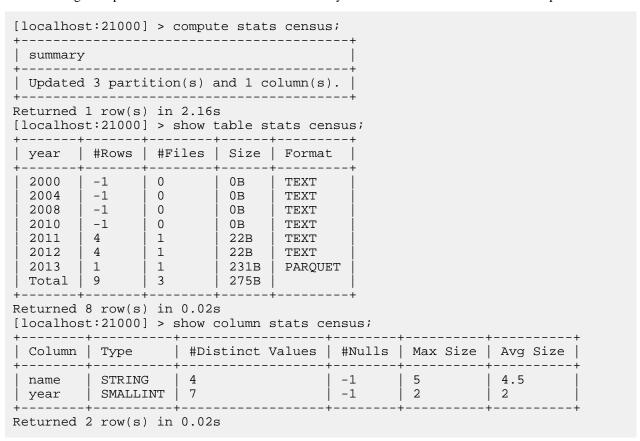
You can see how Impala executes a query differently in each case by observing the EXPLAIN output before and after collecting statistics. Measure the before and after query times, and examine the throughput numbers in before and after SUMMARY or PROFILE output, to verify how much the improved plan speeds up performance.
