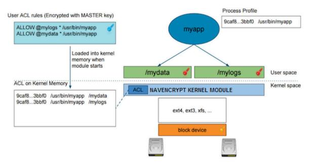
The user adds a rule to allow /usr/bin/myapp to access the encrypted data in the category @mylogs, and adds another rule to allow /usr/bin/myapp to access encrypted data in the category @mydata. These two rules are loaded into the navencrypt-kernel-module cache after restarting the kernel module.
