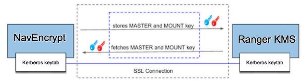
The master key is encrypted by Navigator Encrypt using a local GPG key and stored in the Ranger KMS database. When the master key is needed to perform a Navigator Encrypt operation, Navigator Encrypt fetches the key from Ranger KMS and decrypts the key using the local GPG key.
