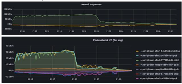
In the second half of the test all agents are registered, and only lightweight heartbeats are sent. Output traffic rate is lower than 10 MB/s at the peak.
