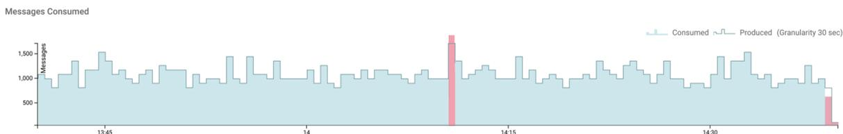
In the preceding image, the linear formation represents the number of messages produced in last one hour, and the filled area represents the number of messages consumed in last one hour with a granularity of 30 seconds. The blue area signifies that all the produced messages are consumed. The red area represents a discrepancy in the produced and consumed message count and can either mean that messages are overconsumed or underconsumed.
