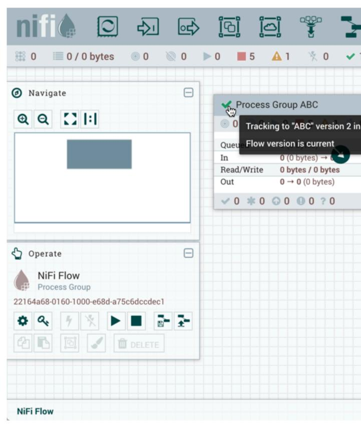
In the example shown, the versioned flow is upgraded from an older to the newer latest version. However, a versioned flow can also be rollbacked to an older version.
