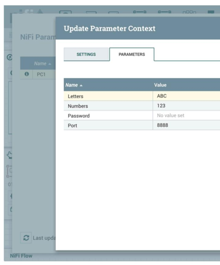
The "Letters" parameter did not exist in the NiFi instance and was added. The "Numbers" parameter existed in both the versioned flow and NiFi instance with identical values, so no changes were made. "Password" is a sensitive
