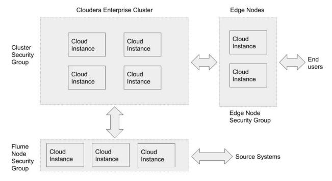
Source systems are where the data is being ingested from using Flume. You'll have Flume sources deployed on those machines.
