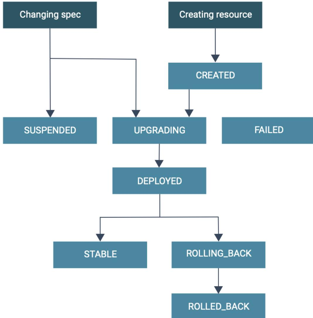
As the Flink Operator is responsible to manage the lifecycle of Flink applications, the behavior of the Flink Operator is controlled by the respective configuration property of the `spec.job` in the `FlinkDeployment` and `FlinkSessionJob` resources.
