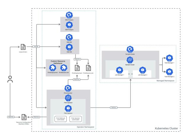
When installing the CSA Operator with Helm, the Flink Operator Webhook is also installed as a custom admission plugin, which allows dynamic admission control. Similarly to connectors, you can use it to add plugins to the Flink operator that add custom rules triggered by certain actions.
