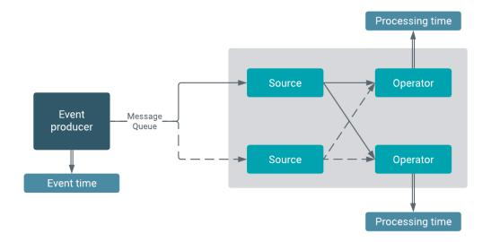
With only the event time, it is not clear when the events are processed in the application. To track the time for an event time based application, watermark can be used.
