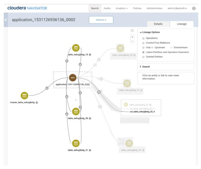
Figure 6: Column Filtering for Spark Lineage Identifies Contributing Assets
