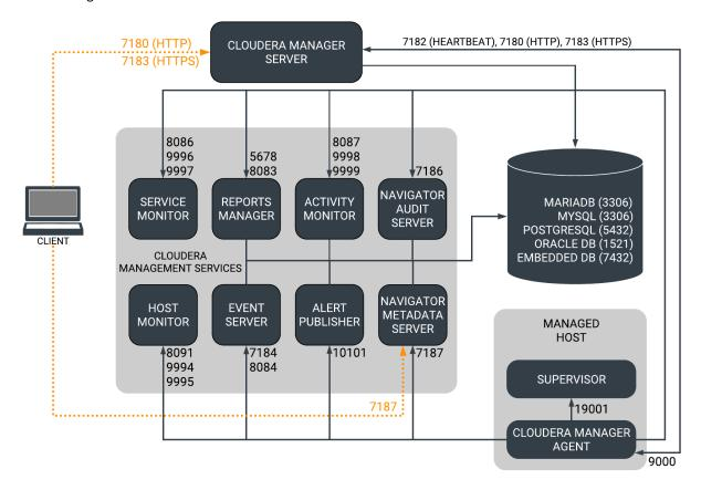
Figure 1: Ports Used by Cloudera Manager and Cloudera Navigator
