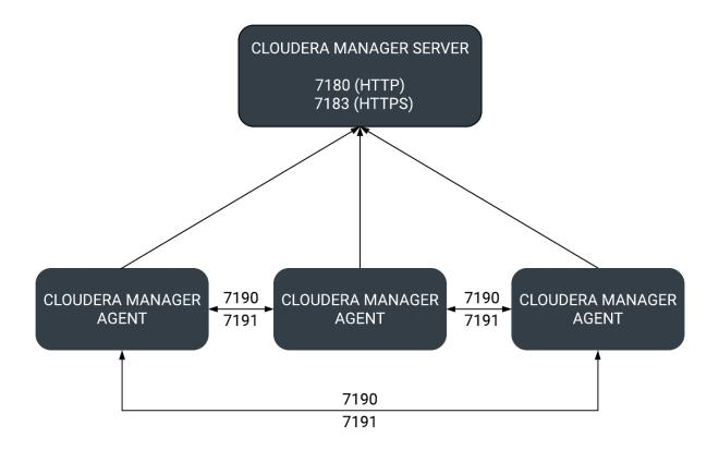
Figure 2: Ports Used in Peer-to-Peer Parcel Distribution
