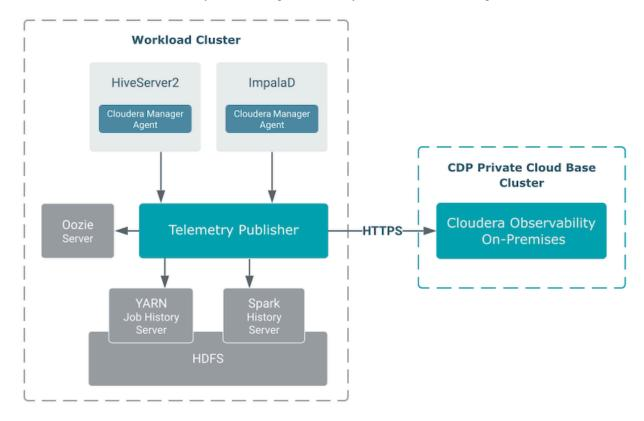
Telemetry Publisher collects and transmits metrics as well as configuration and log files from Impala, Oozie, Hive, YARN, and Spark services for jobs running on your clusters to Cloudera Observability On-Premises, as shown in the above diagram. The metrics are collected as follows:
