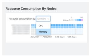
• The Memory Utilization chart widget, displays the aggregated maximum amount of memory that is used by the queries on any node performing the processing. It helps you identify inefficient queries that are consuming the most amount of memory and decide if you need to allocate more memory to continue running your query jobs.
