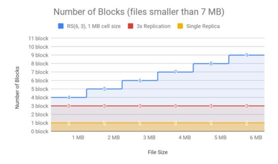
As shown in the following figure, the RS(6,3) EC policy ensures that the number of data blocks continues to remain less than that used by 3x replication for larger file sizes.
