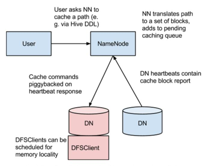
The NameNode queries its set of cache directives to determine which paths should be cached. Cache directives are persistently stored in the fsimage and edit logs, and can be added, removed, and modified through Java and command-line APIs. The NameNode also stores a set of cache pools, which are administrative entities used to group cache directives together for resource management, and to enforce permissions.
