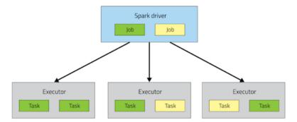
Invoking an action inside a Spark application triggers the launch of a *job* to fulfill it. Spark examines the dataset on which that action depends and formulates an execution plan. The execution plan assembles the dataset transformations into stages. A *stage* is a collection of tasks that run the same code, each on a different subset of the data.
