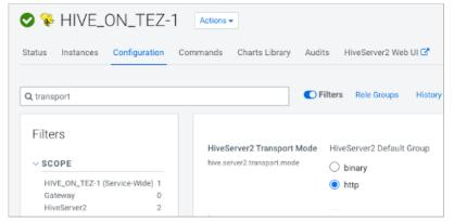
KNOX discovers the service automatically and builds a proxy URL for Hive on Tez only when the transport mode is http.
