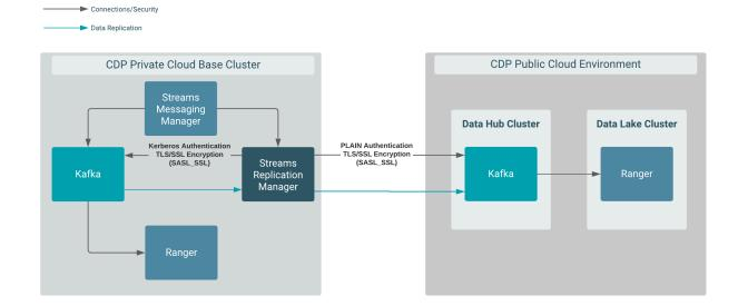
In this scenario, data is replicated from a CDP PvC Base cluster that has Kafka, SRM, and SMM deployed on it. This is a secure cluster that has TLS/SSL encryption and Kerberos authentication enabled. In addition, it uses Ranger for authorization.
