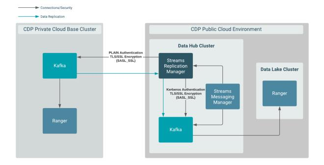
In this scenario, data is replicated from a CDP PvC Base cluster to a Data Hub cluster by an SRM instance that is deployed in the Data Hub cluster.
