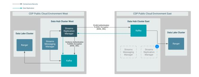
In this scenario, data is replicated between two Data Hub clusters that are provisioned in different CDP environments. More specifically, data in Data Hub East is replicated to Data Hub West by an instance of SRM running in Data Hub West.
