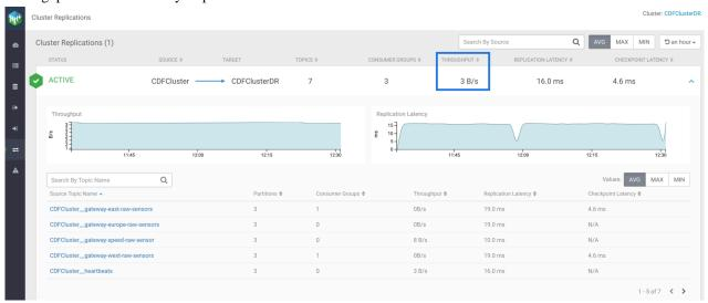
In the image, you can see the average throughput for the CDFCluster to CDFClusterDR replication is 3 bytes per second. You can fetch the maximum or minimum throughput for the replication by clicking the MAX or MIN button located above the cluster replication.
