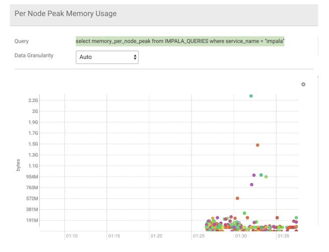
This type of chart can be used to determine the memory limits for a particular pool. Note that most queries use less than 1.2 GB per node. See Admission Control and Query Queuing for more information about Impala admission control.
