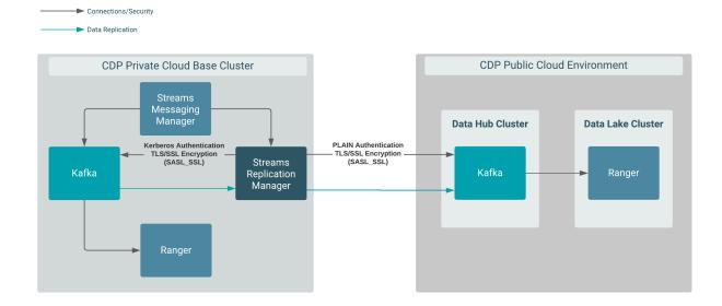
In this scenario, data is replicated from a CDP PvC Base cluster that has Kafka, SRM, and SMM deployed on it. This is a secure cluster that has TLS/SSL encryption and Kerberos authentication enabled. In addition, it uses Ranger for authorization.
